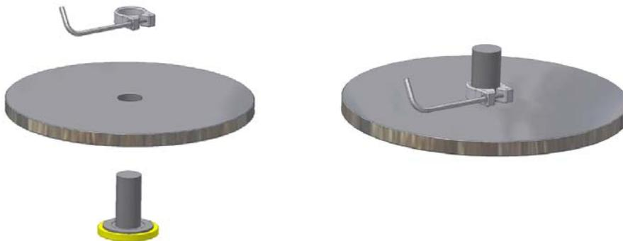
**Pic. 4:** Connection sub-platter and bearing upper part
