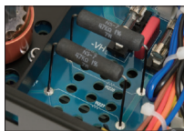
Non-inductive winding resistor with least inductance made by VISHAY Co. (700T)
