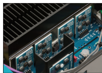
The power transistor array with effective heat dissipation through large-sized heat sink (700S)
