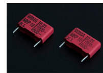
High-definition film capacitor made by German WIMA is used (common to 700T and 700S)
