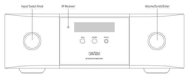
The  $N^05805$  /  $N^05802$  was designed for elegant simplicity and ergonomics. Therefore the knobs perform a variety of functions depending on the operating mode. There are two modes of operation, Listening mode and Setup mode, and three modes of standby, Green, Power-save, and Normal.
