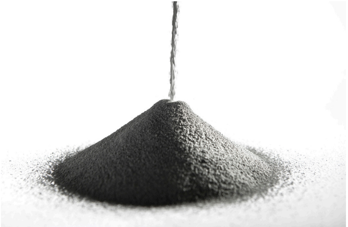
The fine grain SMC material is an important building material in the materialization of the high performance EPICON magnet system.
